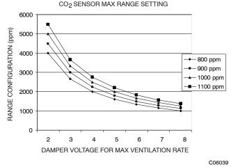
Fig. 82 - CO<sub>2</sub> Sensor Maximum Range Settings
